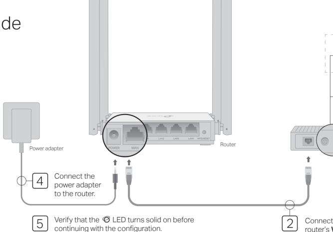
Connect the powered-off modem to the router's **WAN** port via an Ethernet cable.
